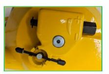
**Drum Lock System** Drum lock for cable replacement
