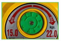
Gauge Indicator for recognition on tension adjustment
